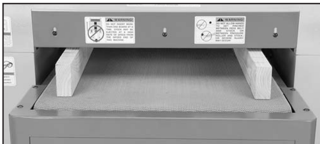
Figure 63. 2x4s placed on feed belt under sanding drum.
